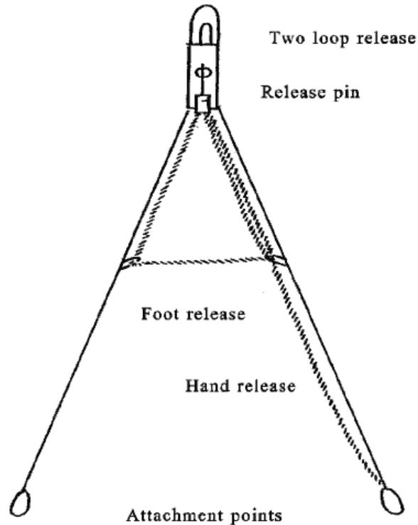
Figure 2 – “Hystek” Paraglider release and bridle - top elevation
