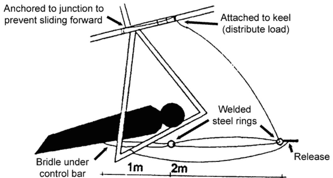
Where a release system releases a tow bridle from the keel, a weak link must be attached to the pilot
