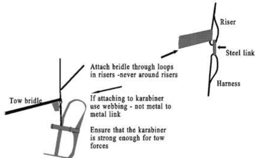
When the bridle is connected to the risers it is preferable to fit it to the loop in the riser to ensure that it cannot slide up the riser.
