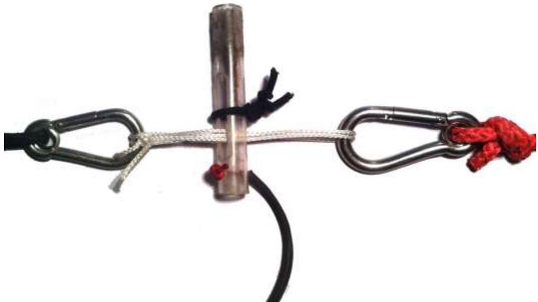
Figure 3 - Link Knife. In this photo, the o-ring has been replaced by a bungey cord.
