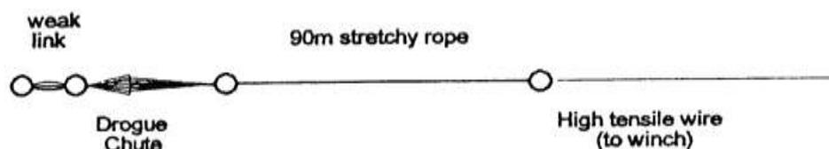
Prior to use, ropes should be stretched out on the ground and inspected for knots and wear. Unnecessary knots should be removed and worn lines replaced.
